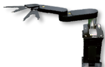
For wafer transfer N & T Series (clean)
