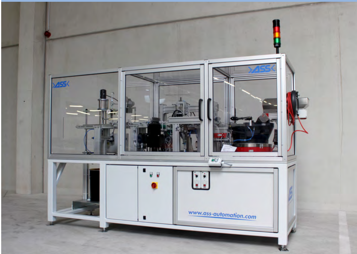
Automation system with processing, assembly and testing tasks
