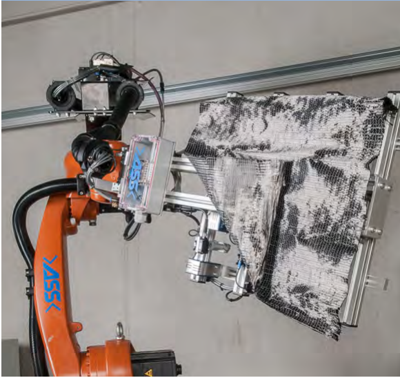
Handling of CFRP
