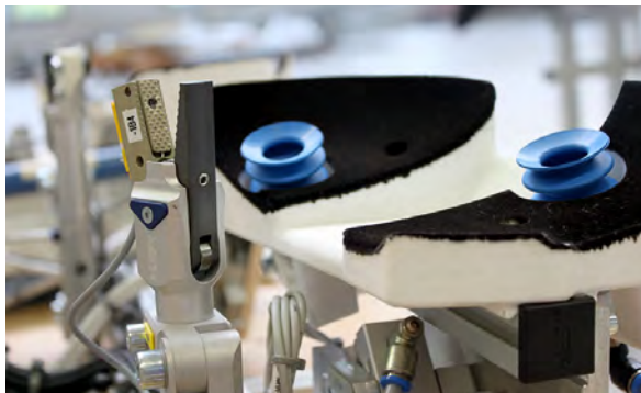
Flocked counter piece for a very soft discard for sensible parts
