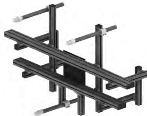
Frame for bumper coat cavity site de-molding
